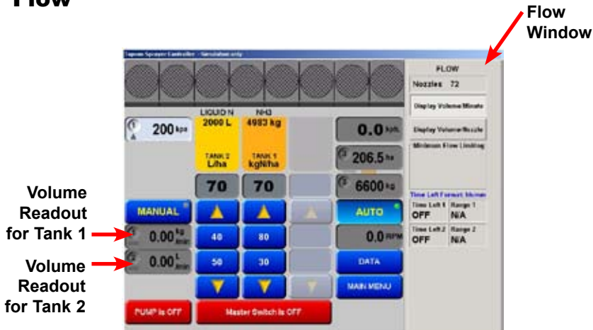
Figure 10-2. Working Screen Showing Flow Window
